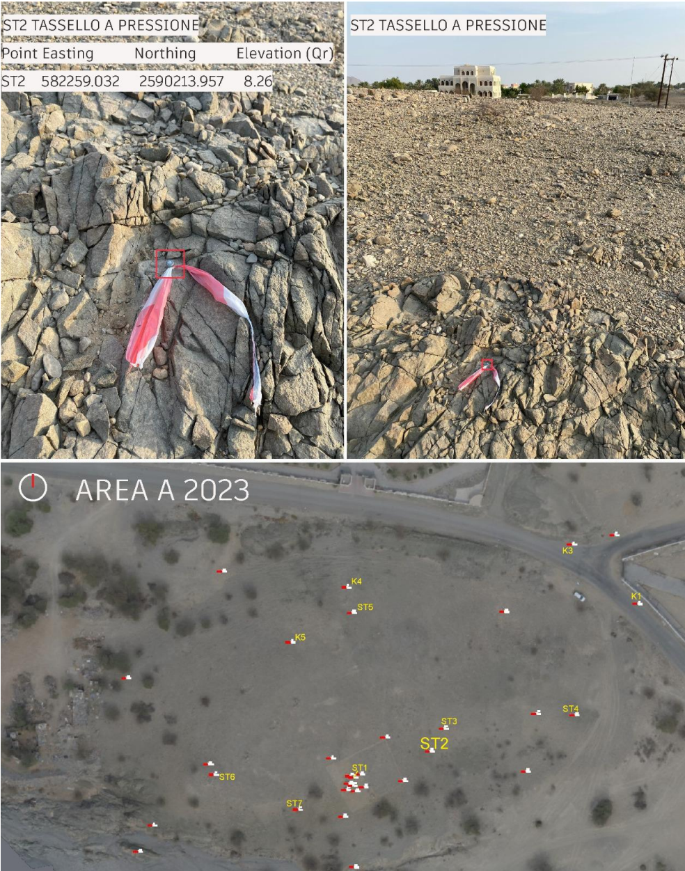
Fig. 14.1. Area A, Wadi al-Ma'awil, the I Order topographic network (Photo shooting and processing D. Rose and C. Schiatti, ©MASPAG, courtesy MHT).
