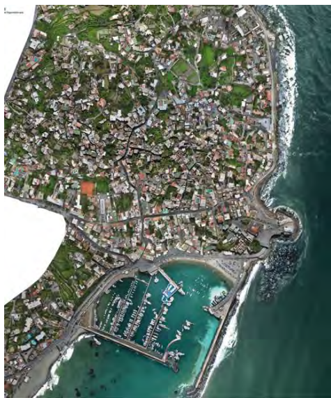
Fig. 8- Ortomosaico, 52.871 × 6.434 pixel, 2.06 cm/pixel (GSD), scala 1:200 (Patryk Rynkowski, 2024)
