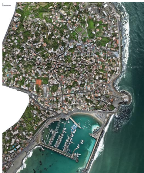
Fig. 8- Ortomosaico, 52.871 × 6.434 pixel, 2.06 cm/pixel (GSD), scala 1:200 (Patryk Rynkowski, 2024)
