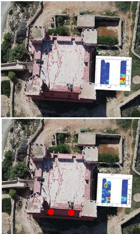
Fig. 4- GPR slices close to the Red Tower. On the GPR slices close to the Red Tower. At the top: depth of about 70 cm. At the bottom: depth of about 100 cm. The red dots indicate the plaster sampling points
