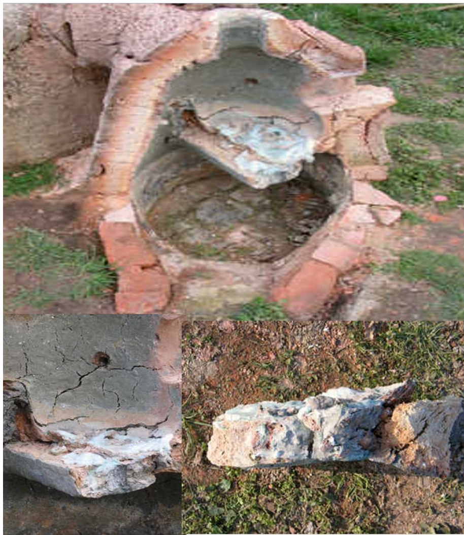
Fig. 10.10. The dismantling of a roman tank-furnace replica with particular of the bottom of the tank with a layer of glass attached to the clayey material (elaboration by the author; credit Roman Furnace Project 2006, http://www.theglassmakers.co.uk/archiveromanglassmakers/furnace27.htm ).
